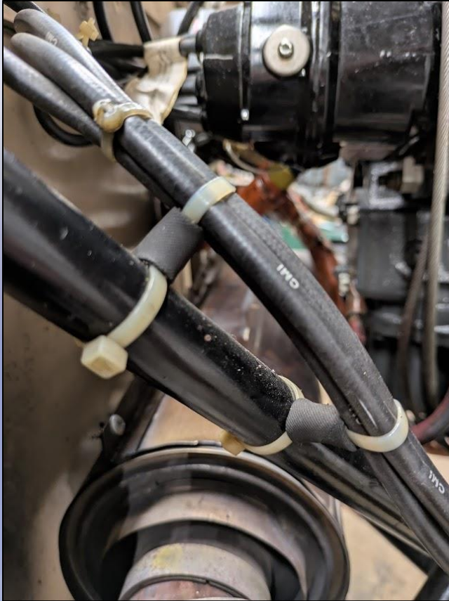
Standoffs for High Temperature And Vibration Areas
