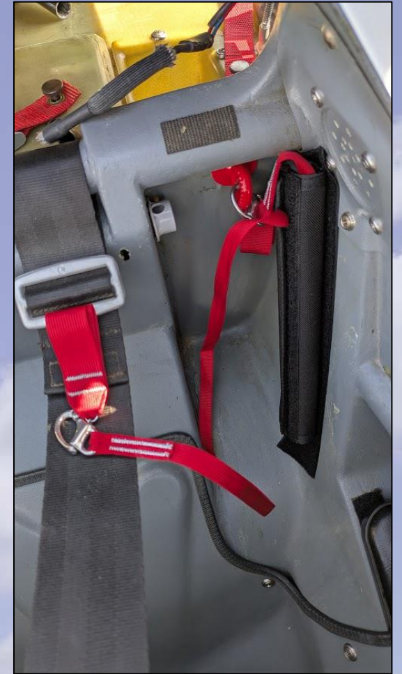
Style #2 - Static Line container mounted inside the glider
